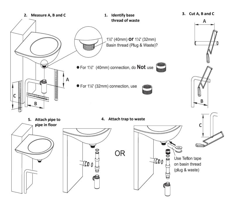
If trap is going into a 40mm socket, use key seal (included in box). If trap is going into 40mm pipe, push straight in and seal with silicone.
