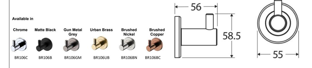
We aim to ensure the specifications are correct at the time of publication. Always use measurements of the actual product received for the final specifications as there may be slight differences with the drawing shown. All measurements are in millimetres
